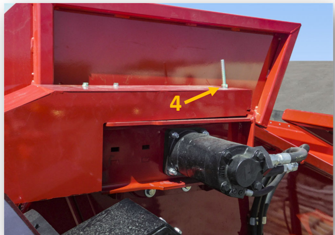
Figure 8-27: Drive Motor Chain Tension
