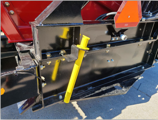
Figure 8-3: Tank Safety Pin Storage Location
