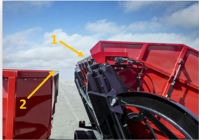
Figure 6-2: Tank Distance from Receiving Unit
