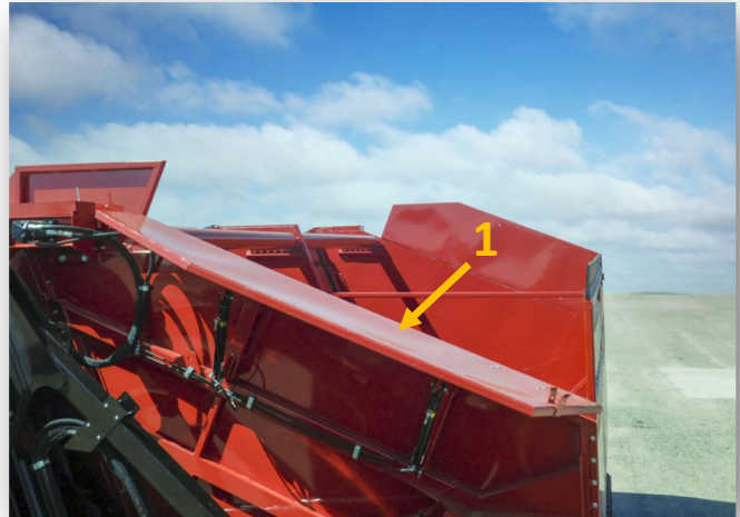
Figure 6-1: Front Top Gate in Lowered Position
