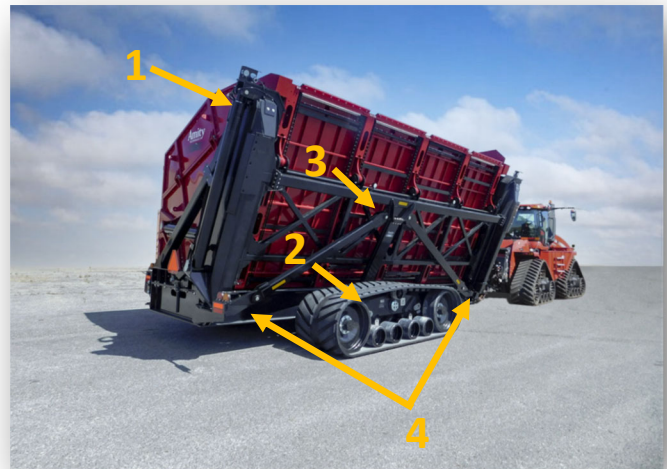
Figure 8-1: Areas of Debris Buildup
