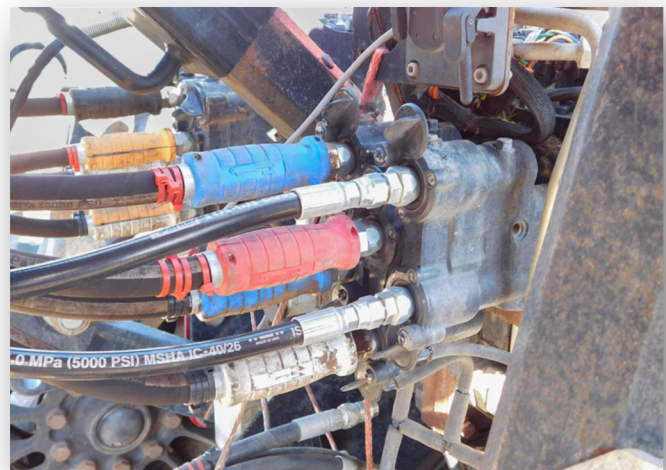
Figure 5-2: Attaching Hydraulic Hoses
