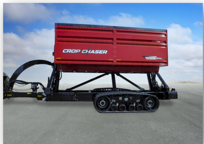
Figure 8-2: Tank Raised for Cleaning
