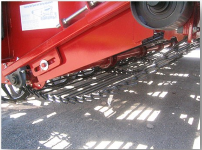
Figure 9-4: Apron Shaft Cleaning
