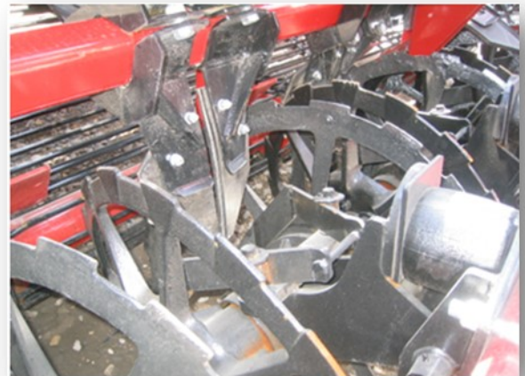
Figure 9-2: Lifter Strut and Paddle Cleaning
