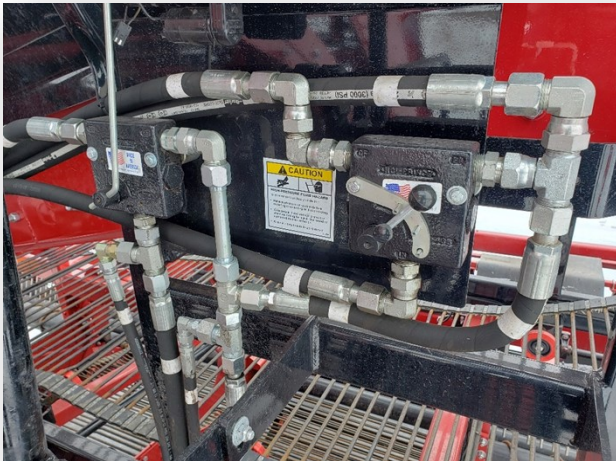
Figure 7-35: Scrub Chain Flow Control Valves
