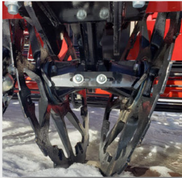
Figure 6-8: Scrapper, Single Plate Strut
