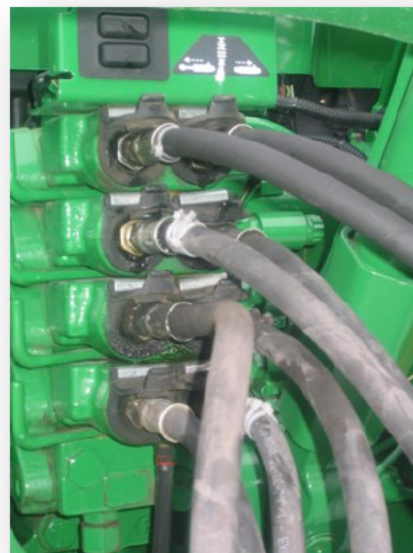
Figure 5-1: Attaching Hydraulic Lines
