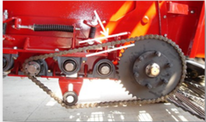
Figure 7-34: Jump Chain Tension
