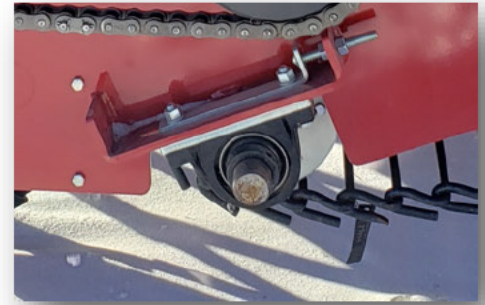
Figure 7-19: Apron Chain Front Idler Shaft
