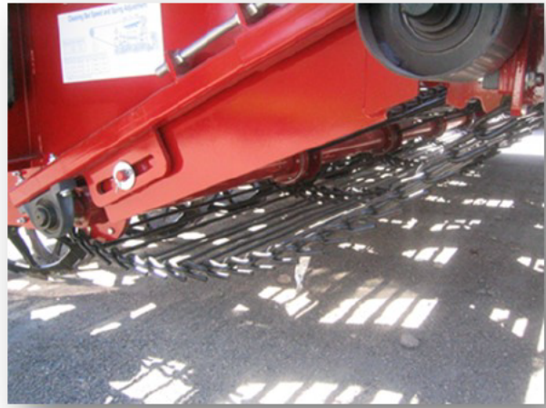
Figure 9-4: Apron Shaft Cleaning
