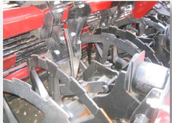
Figure 9-2: Lifter Strut and Paddle Cleaning
