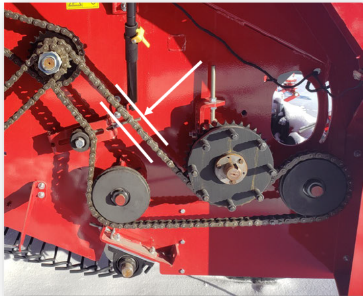
Figure 7-33: Paddle Shaft Chain Tension
