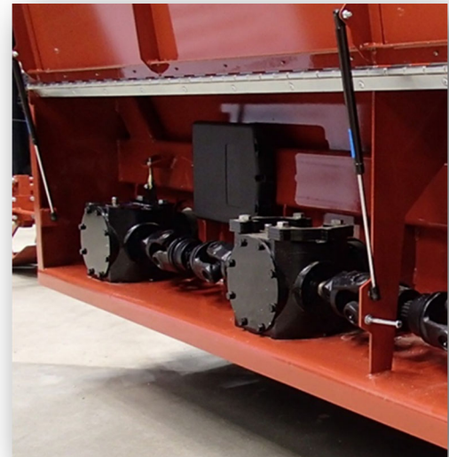
Figure 7-5: Gearbox 3 rd Drum Adjustment
