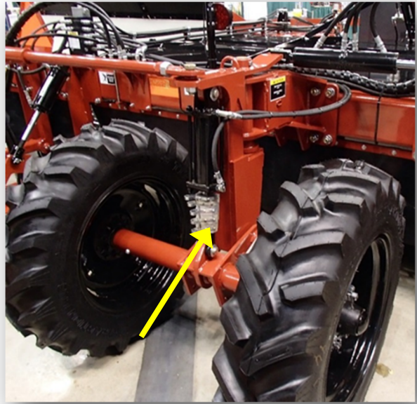
Figure 7-2: Rear Strut Height Adjustment
